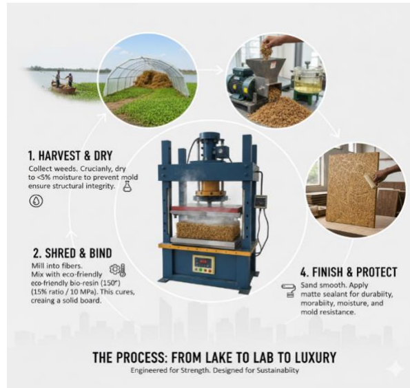
Fig. 1. Schematic outline of the proposed circular-economy process for converting invasive aquatic weed biomass into value-added composite Lake Board panels.
