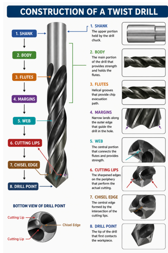
Figure 2.1 Construction of a Twist Drill
