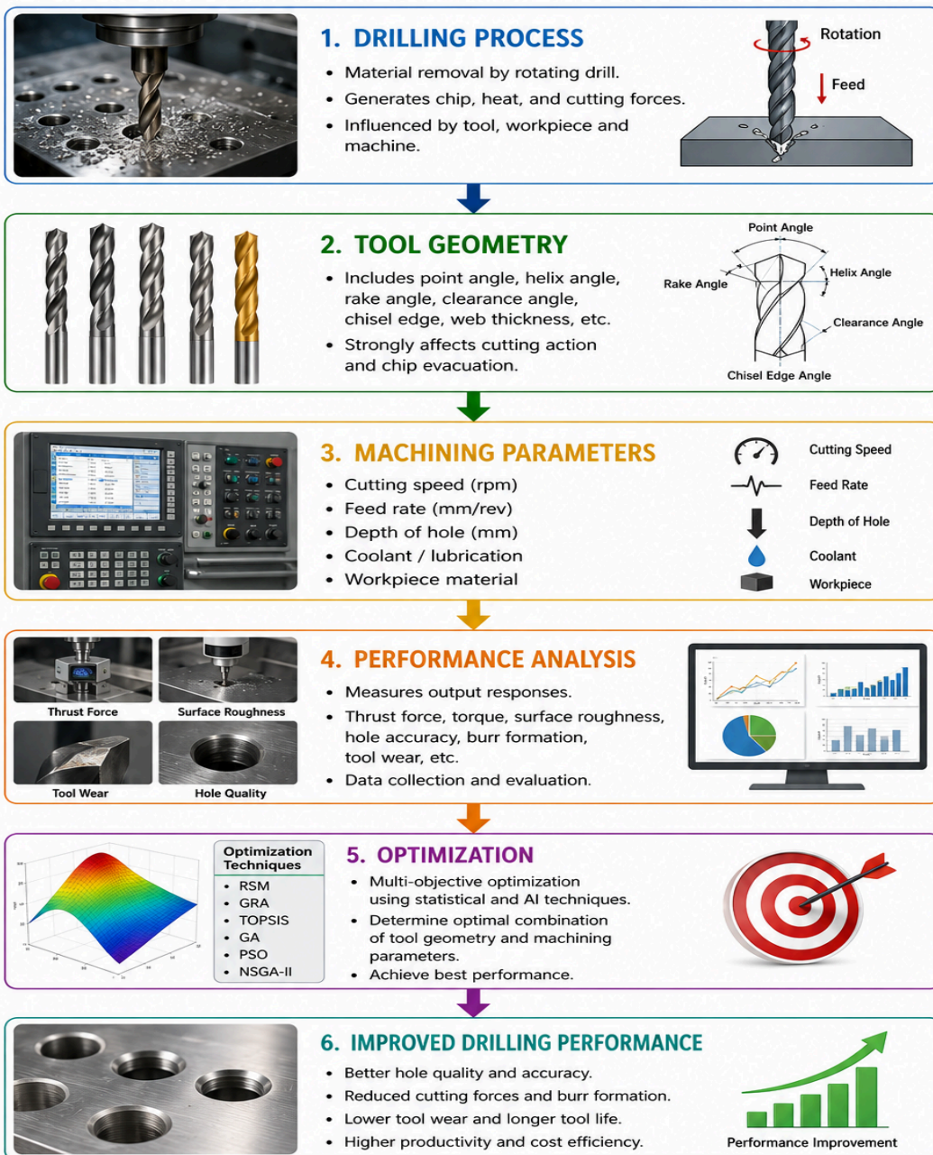
Figure 1.1 Overall Framework of Drilling Tool Geometry Optimization
