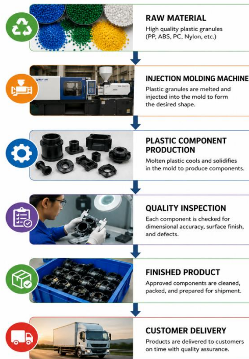
Figure 1.1: Overall manufacturing framework of plastic injection molding industries showing the transformation of raw materials into finished products through molding operations.
