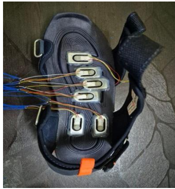
Fig 3.2 Half-Bridge Load Cell Sensor
