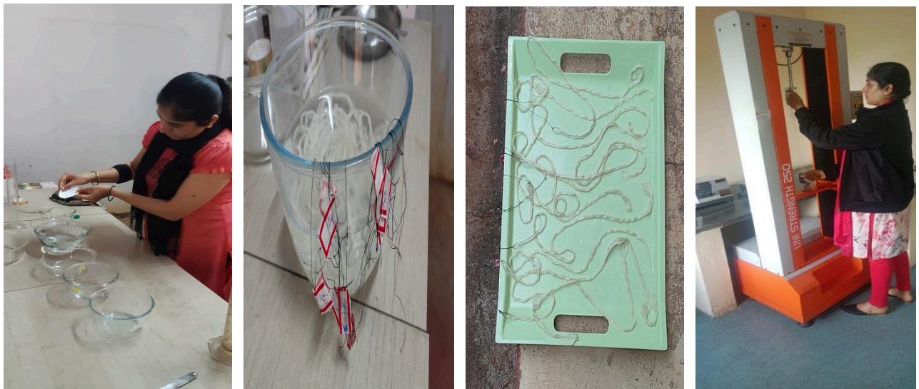
Fig.2.1 Application of polyacrylamide on silk filaments and testing of treated silk filaments
